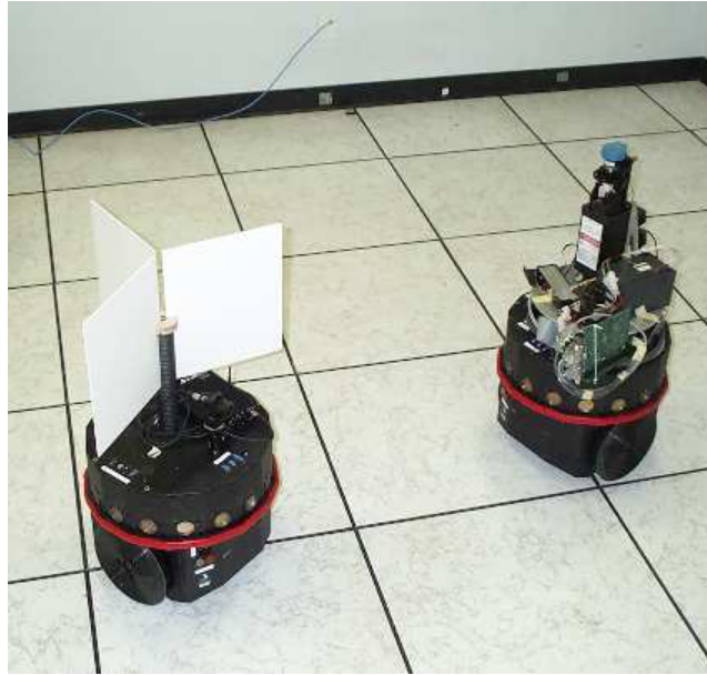
Figure 11: Robots employed for data collection. The three-plane target mounted on the exploring robot is sensed by the stationary robot, allowing for the computation of pose estimates for the explorer. The pose estimates are employed as an approximation to ground-truth, both for training and evaluating the vision-based localizer.
