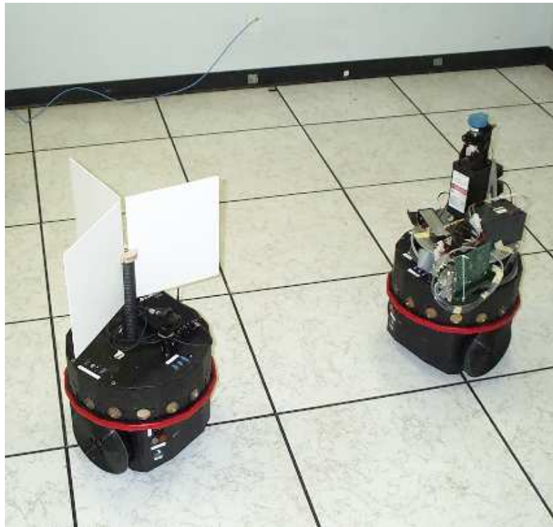
FIGURE 3.10. Robots employed for data collection. The three-plane target mounted on the exploring robot is sensed by the stationary robot, allowing for the computation of pose estimates for the explorer. The pose estimates are employed as an approximation to ground-truth, both for training and evaluating the vision-based localizer.
