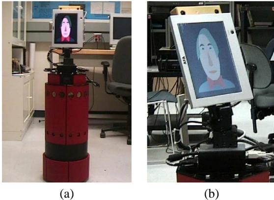
Fig. 2. The RWI B14 robot we used for data collection as (a) seen from a distance and (b) closeup of its head.
