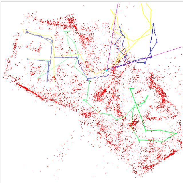
Fig. 5. The constructed map based solely on the visual odometry.
