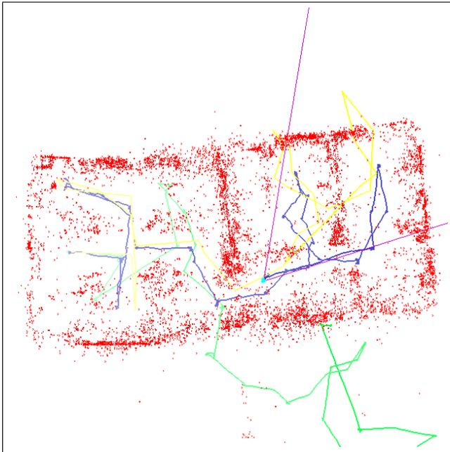
Fig. 4. The constructed map for the best sample at the end of exploration. The blue trajectory indicates the trajectory of the best sample and the green trajectory indicates the visual odometry measurements. The robot odometer (not used for map estimation) is plotted as a yellow trajectory. Landmark positions are marked with red 'X's. The set of particles is shown by the cyan blob near the center. The width of the map is approximately 18m.
