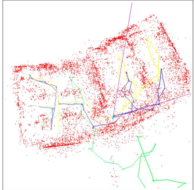
Fig. 6. The constructed map based solely on the robot's odometer (which was not used for constructing the map in Figure 4).
