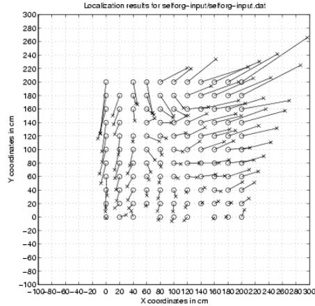
Figure 2: Self-organizing pose estimates plotted versus ground truth for the LAB scene.
