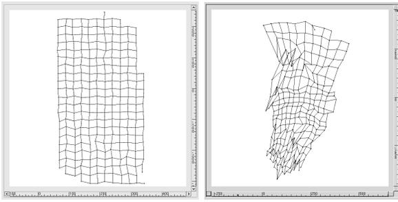
Figure 7: Ground truth, and the map resulting from the self-organizing process for the environment depicted in Figure 1.
