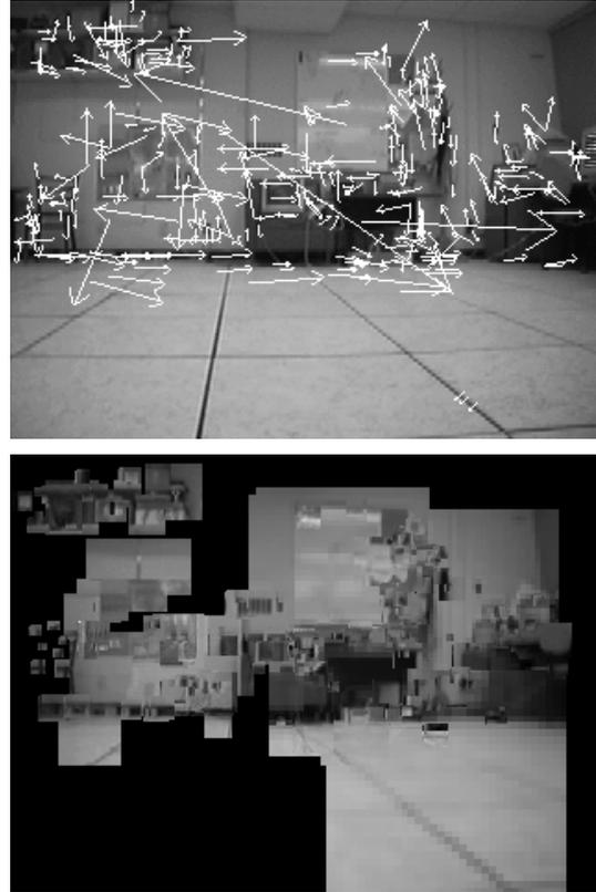
Fig. 1. a) Detected SIFT features in an image. Each arrow corresponds to a detected feature, with scale corresponding to arrow length, and orientation corresponding to arrow direction. b) Modeled SIFT features rendered from a novel viewpoint.
